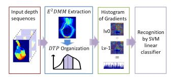
Figure 1. Flowchart of proposed approach. After edge enhanced depth motion map extraction and dynamic temporal pyramid (DT-P) organization, we apply Histogram of Gradients (HoG) to generate vectored representation of the two levels of  $E^2DMM$  (lv0 and lv-1). Finally, a SVM classifier is trained and utilized for classification.
