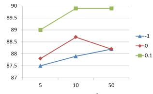
Figure 6. Performance evaluation of  $E^2DMM$  on dynamic hand gesture dataset [9] of different parameter settings. X axis: penetration threshold  $\epsilon$ ; Y axis: performance in term of classification accuracy. Blue, red and green colored curves indicate degree of enhancement -1, 0, and 0.1 respectively. Notice that when degree of enhancement is -1, it actually represents traditional DMM [16].
