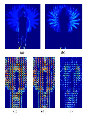
Figure 2. Illustration of edge suppression in DMM [16] computation of action "Two Hands Wave" in [8]. (a) DMM without edge suppression. (b) DMM after edge suppression in Equation 1. (c) and (d) are Visualizations of HoG Representations of (a) and (b), respectively. (e) is the difference in feature space of (c) and (d) . The contour of human body can be obviously observed without edge suppression, which causes ambiguity as shown in (e).
