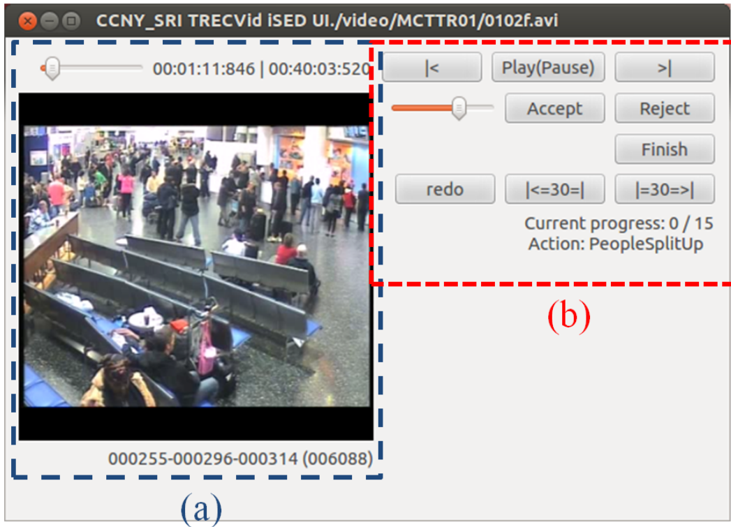
Figure 5: Our Graphical User Interface and functional panels implemented by PyQt4, a cross-platform framework. (a) Video playing and information panel. (b) Control and event information panel.
