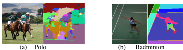
Figure 3. Segmentation examples of two scene images. Pixels with the same color belong to the same segment.
