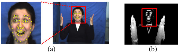
Figure 3: (a) ASM facial landmark points tracking; (b) MHI Image
