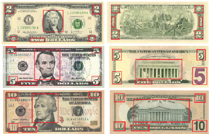
Figure 3: Examples of reference regions with class-specific features on the bills of $2, $5, and $10. Each region marked in red box is one reference region.
