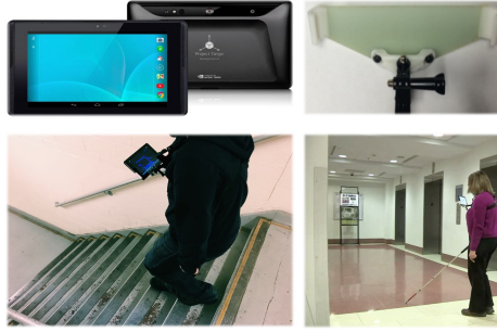
Fig. 3. The basic hardware configuration of the proposed assistive navigation system, including the Google Tango Tablet device and the 3D printed chest level tablet mount.
