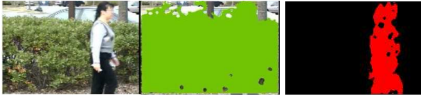
Figure 4: A person moving in front of wind-blown foliage. Centre: the result of a conventional background subtraction algorithm. Right: The object detected using salient motion. Background subtraction and salient motion detection are complementary approaches. Background subtraction is more suited for indoor environments where lighting is fairly stable and distracting motions are limited, whereas salient motion detection is well suited to detection in outdoor situations.
