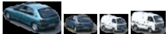
Figure 5: Appearance models from a PETS 2001 [2] video sequence, showing the appearance of model pixels, as one model recedes (left) and another approaches (right). Pixels not in the model appear black.
