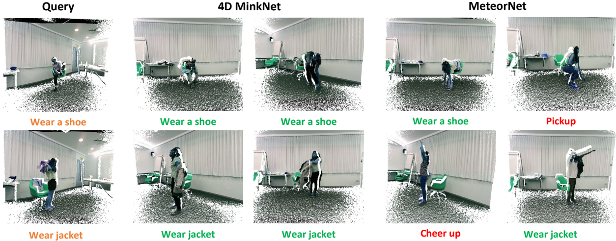
Figure 4. Demonstraton of top2 accuracy for nearest neighbor retrieval. The center frame is used to represent the point cloud sequence. The first column represent query clips from the testing split,the middle and last two columns show the result with 4D MinkNnet and the MeteorNet respectively.
