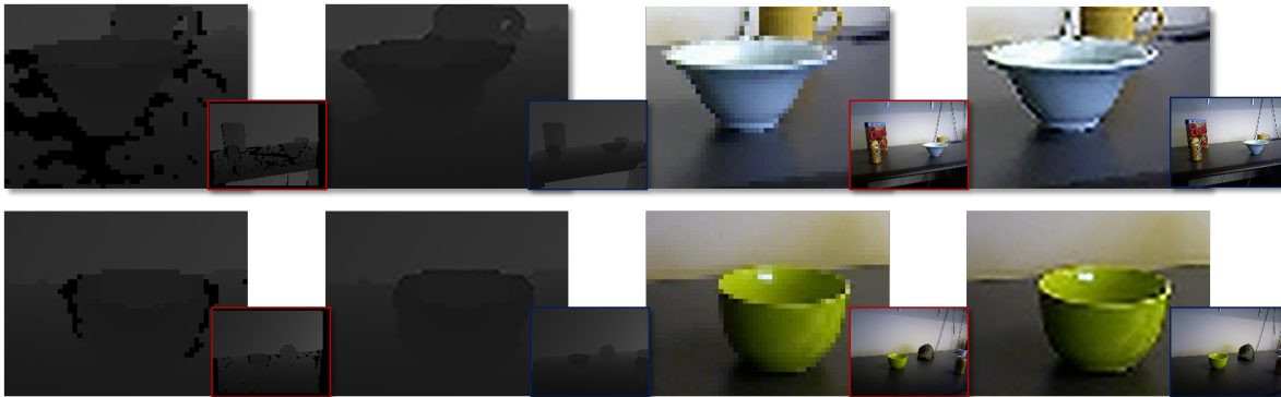
Figure 5. Resolution enhancement results in RGBD Scenes dataset v2 [17] ( \times 4 ). From left to right, the columns represent LR input depth maps, generated HR depth maps, LR intensity images, and HR intensity outputs. For a better presentation, the input instances are upsampled through nearest-neighbor interpolation. This figure is better viewed on screen with HR display.
