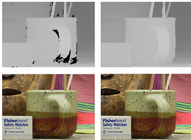
Figure 1. Enhancement results of 'cone' (partial) ( \times 4 ). Left column present the low-resolution depth map and the intensity image while the right column are the corresponding high-resolution results generated by the proposed enhancement framework. The LR instances are upsampled by nearest-neighbor interpolation for a better illustration. The figure is better viewed on screen with HR display.
