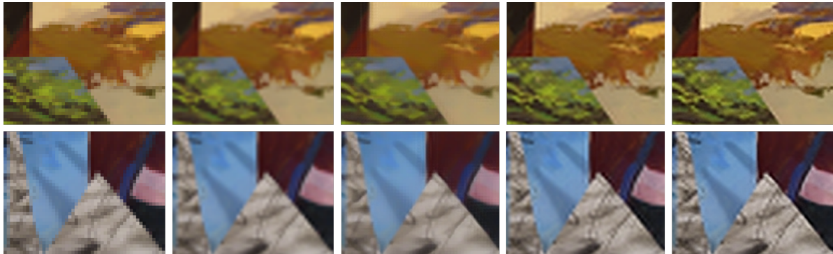
Figure 7. SR results of RGB images ‘bull’ and ‘sawtooth’ ( \times 4 ). From left to right, the columns represent the results generated through nearest-neighbor interpolation, bicubic interpolation, ScSR [36], GR [32], and the proposed system. Only partial of the images are shown for a clearer presentation. The figure is better viewed on screen with HR display.
