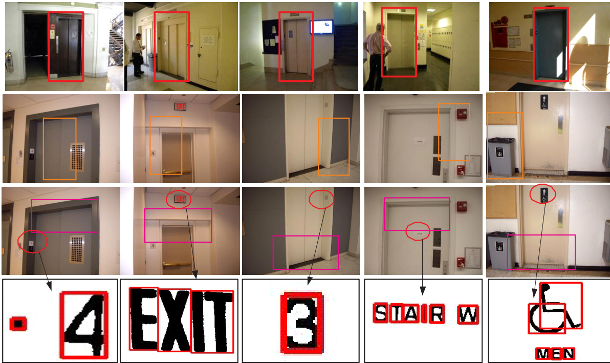
Figure 6. Examples of detection results. The first row shows examples of successful detection results according to the first layer decomposition models. The second row shows failed cases by only using the first layer model but which can be correctly detected by using the second layer models. The fourth row shows the extracted contextual information which help model decomposition
