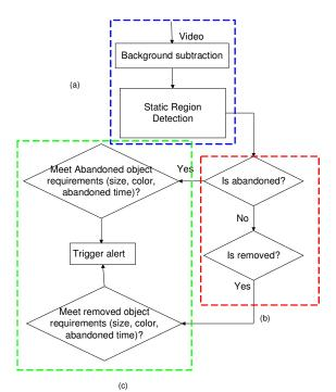
Figure 1: System diagram: (a) background subtraction and static region detection; (b) object type detection (abandoned or removed); (c) abandoned and removed object alert detection.
