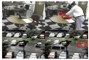
Figure 7 – Examples of detected removed objects.
