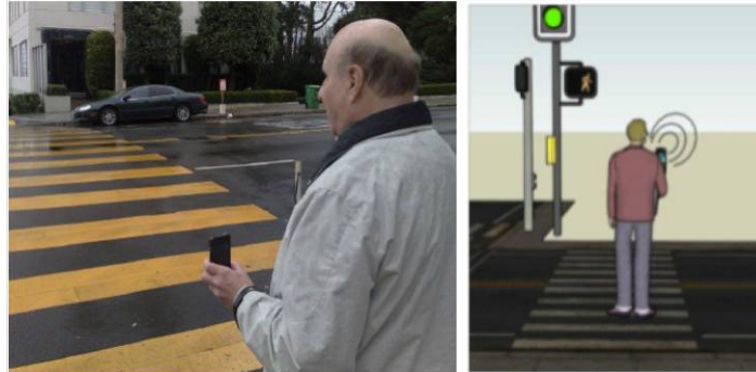
Figure 2: Crosswatch system for providing guidance to visually impaired pedestrians at traffic intersections by panning a cell phone camera left and right; the system provides feedback to help user align him/herself to crosswalk before entering it [28].
