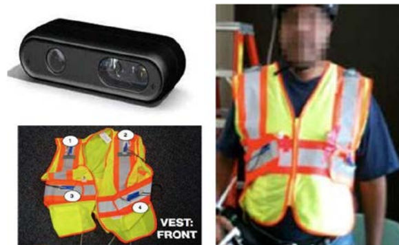
Figure 6. The RGB-D camera based navigation aid for the visually impaired which includes a RGB-D camera and a tactile vest interface device [52].
