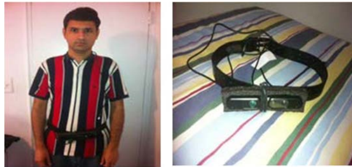
Figure 5. The Xtion Pro Live-Waist assemblies for detecting humans and obstacles [48].
