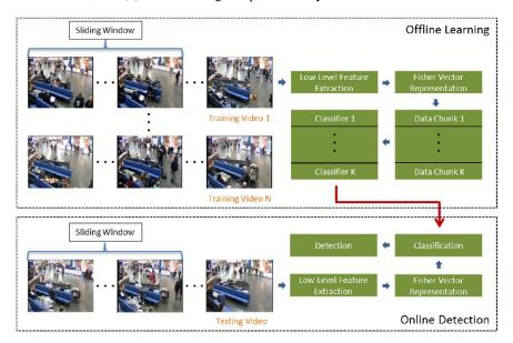
Figure 1: Overview of the CCNY generic surveillance event detection system.
