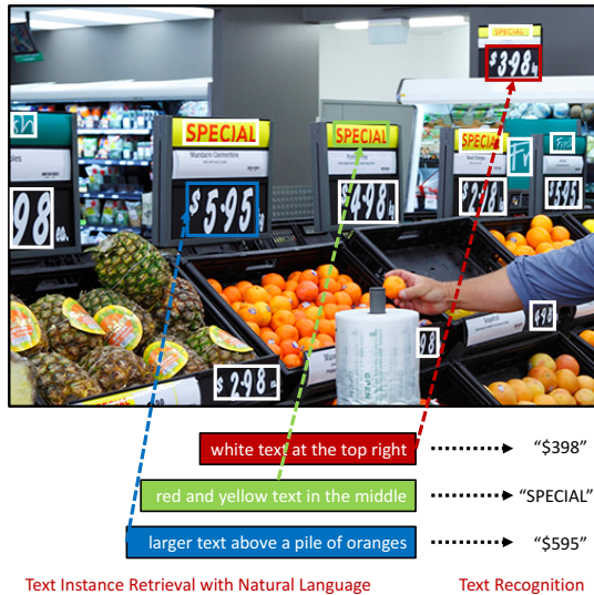
Fig. 1: An example of unambiguous text localization, retrieval, and recognition. Given a cluttered scene image and candidate text bounding boxes (in white, detected by the proposed DTLN), the proposed CRTR model is applied to retrieve a specific text instance (in color) based on a natural language description, which can be further transcribed to machine-readable character codes. The CRTR model scores and ranks candidate boxes based on text attributes, spatial configurations, and context information.
