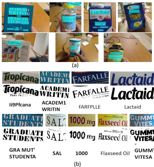
Fig. 16. (a) Some results of text localization on the user-captured dataset, where localized text regions are marked in blue. (b) Two groups of enlarged text regions, binarized text regions, and word recognition results from top to down.
