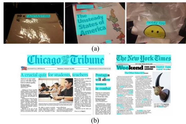
Fig. 4. (a) Our proposed text layout analysis can still be adaptive to oriented text string within reasonable range. (b) The method can handle some challenging cases of font variations, such as newspaper titles.
