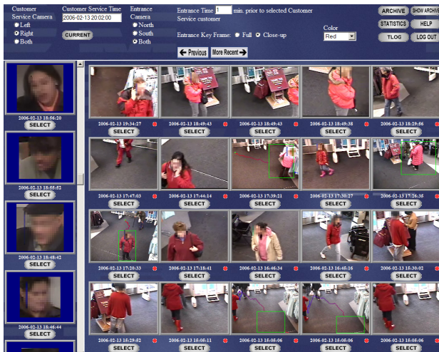
Fig. 3. The user interface is divided into a controls panel (top), customer service events (left) and entrance events (right). These example results are restricted automatically (see Section 4.3 to match the selected “red” search criterion — all matches are wearing red or pink clothing. All faces in this paper are pixellated for privacy.
