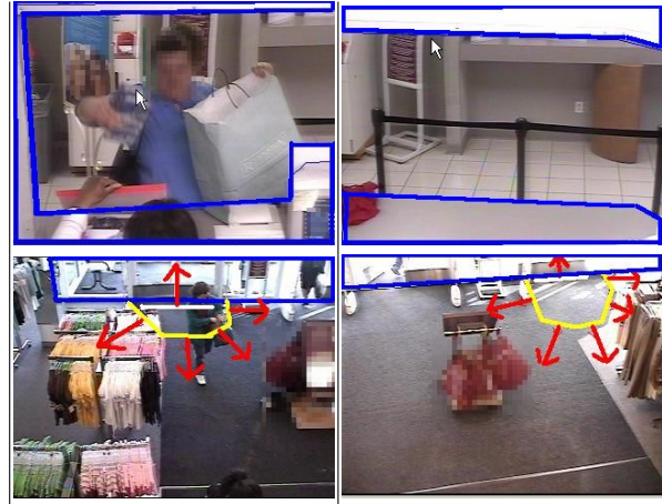
Fig. 2. Views from four of the six cameras — two at the customer service desk (top) and two of the four doors (bottom). The “region of uninterest” is shown in blue for all frames and the entrance tripwires ( enter in yellow, leave in white) are drawn on the views.
