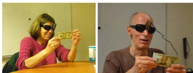
Fig. 8: Evaluation of proposed system by blind subjects. The bill to be recognized is held by hands and image captured by a camera mounted on a pair of sunglasses.
