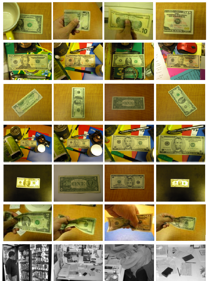
Fig. 7: Training and testing data set of banknote images taken under different conditions and negative images: 1 st row (partial occlusion), 2 nd row (cluttered background), 3 rd row (rotation), 4 th row (scaling change), 5 th row (illumination change), 6 th row (wrinkling), 7 th row (negative images).
