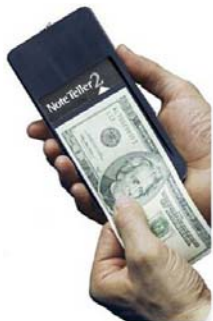
Fig. 2: A portable bill recognition product for blind users in the market “Note Teller 2” [26].
