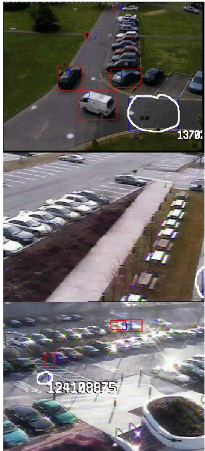
Figure 1 Several examples of different types of track false positives marked in white circles, including (top) track false positives due to a stationary object which begins to move – so called "ghosting," – from PETS 2001 data, (middle) a specular reflection from a glass building not visible in the scene at right and (bottom) due to a strong shadow of a person cast on the road from an extremely bright day.
