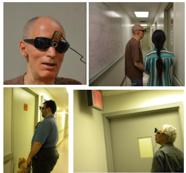
Figure 12. The developed prototype system includes a Logitech web camera with auto focus on sunglasses and tested by blind subjects for signage detection and recognition.
