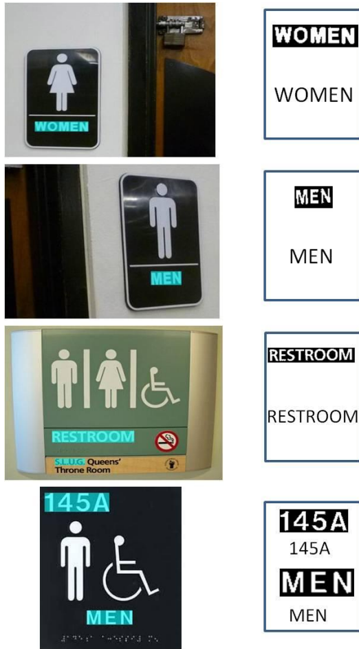
Figure 10. Detected text regions are marked in blue masks in the images (left column). The detected text regions and the corresponding text codes recognized by off-the-shelf OCR are displayed in the right column.
