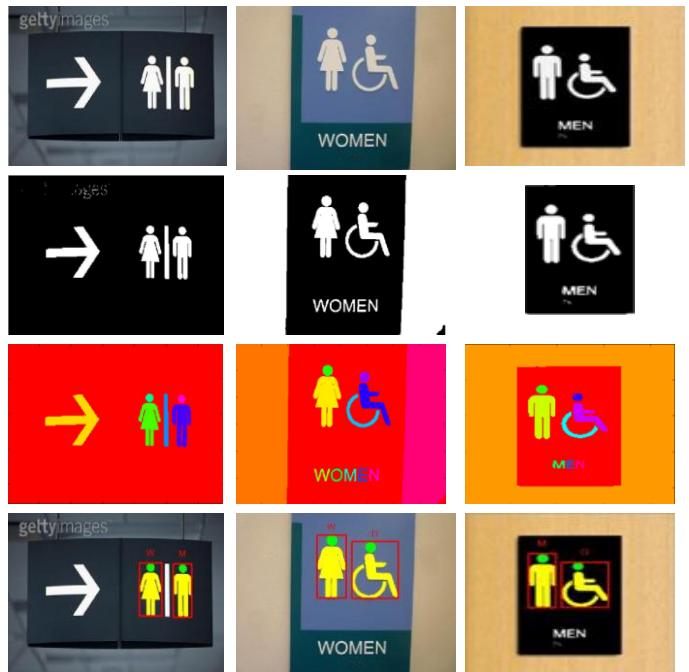
Figure 9. Sample restroom signage images of each step of the proposed method. Rows from top to bottom: original images, binarized images, images with connected components, and detected and recognized signage.
