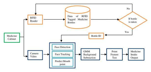
Figure 1. System diagram of the proposed medicine bottle identification by combining video camera and RFID sensors.
