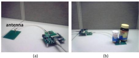
Figure 2. SkyTek M2 RFID system includes a USB connection, antenna, RFID reader, and a host interface board for identifying medicine bottles.
