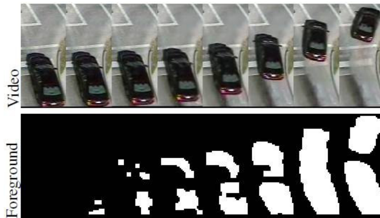
Fig. 5: Selected frames demonstrate ghosting by using mixture of Gaussians BGS. The car starts in the background and moves forward, leading to multiple foreground fragments and ultimately a large “ghost” or “hole” where it had been covering up the “true” background.
