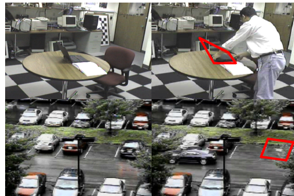
Fig. 13: Examples of detected removed objects in our dataset. The first row shows a moved laptop and the second row demonstrates a parked car driven away.
