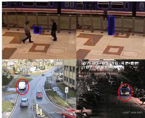
Fig. 12: Examples of the abandoned object detection in complex situations. 1st row: abandoned baggage detection in PETS 2006 dataset [43]. 2nd row: detection of parked cars and abandoned objects in i-LIDS dataset [44].
