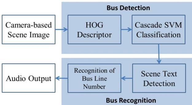
**Fig. 2.** The flowchart of our proposed travelling assistant system for bus detection and recognition.
