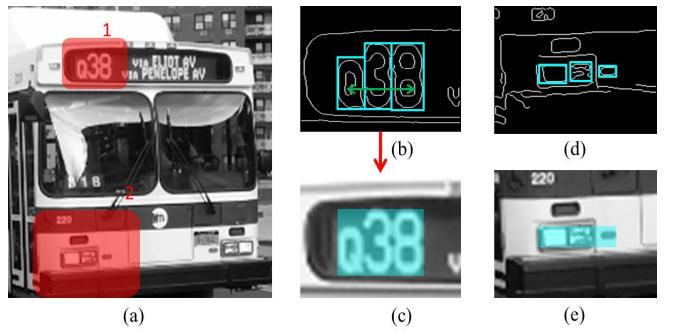
**Fig. 6.** The process of adjacent character grouping. (a) Original image of bus facade with text information. Adjacent groups are obtained in the two shaded regions. (b, d) Finding out three consecutive bounding boxes of candidate character boundaries in edge map. (c, e) An adjacent group in the form of candidate patch.
