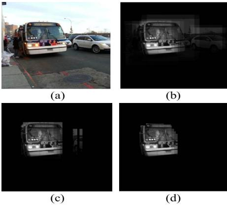
**Fig. 5.** (a) Original image; (b-d) Images after edge-based background filtering with score thresholds at 0, 0.25 and 0.5 respectively.
