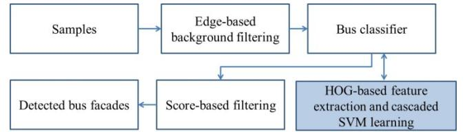
**Fig. 3.** The process of bus detection, including edge-based background filtering and score-based filtering. HOG-based feature extraction is used to train a bus classifier in cascaded SVM model.
