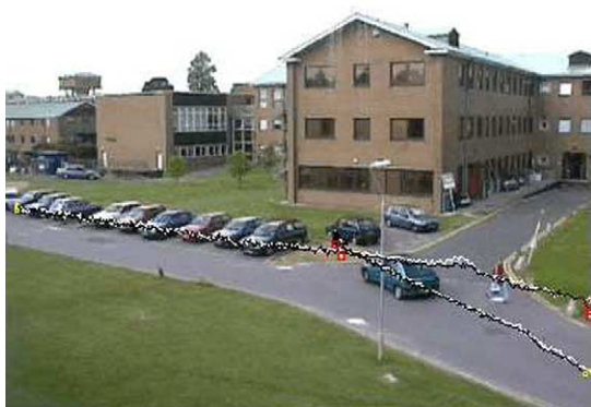
Fig. 8. A comparison of estimated tracks (black) with ground truth positions (white), for two tracks superimposed on a mid-sequence frame showing the two objects.
