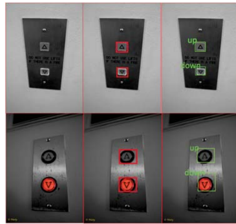
Fig. 10. Elevator Button Label Recognition for outside elevator panels. (a) Input images. (b) Ground-truths of button detection. (c) Results of button recognition.
