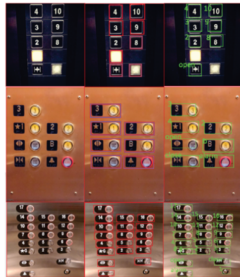
Fig. 11. Elevator Button Label Recognition. (a) Input images. (b) Ground-truths of button detection. (c) Results of button recognition.
