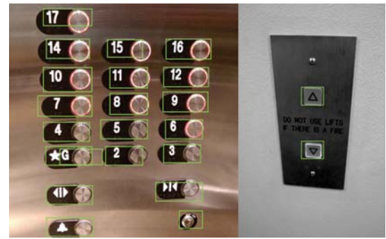
Fig. 5. Examples of the results for pair-wise button and label detection.
