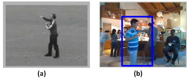
Fig. 1. Comparing the differences between action classification and detection. (a): for a classification task we need only estimate the category label for a given video. (b) for an action detection task we need not only estimate the category of the action but also the location of the action instance. The blue bounding box illustrate a desirable detection. It can be seen that the action detection task is crucial when there is cluttered background and multiple persons in the scene.
