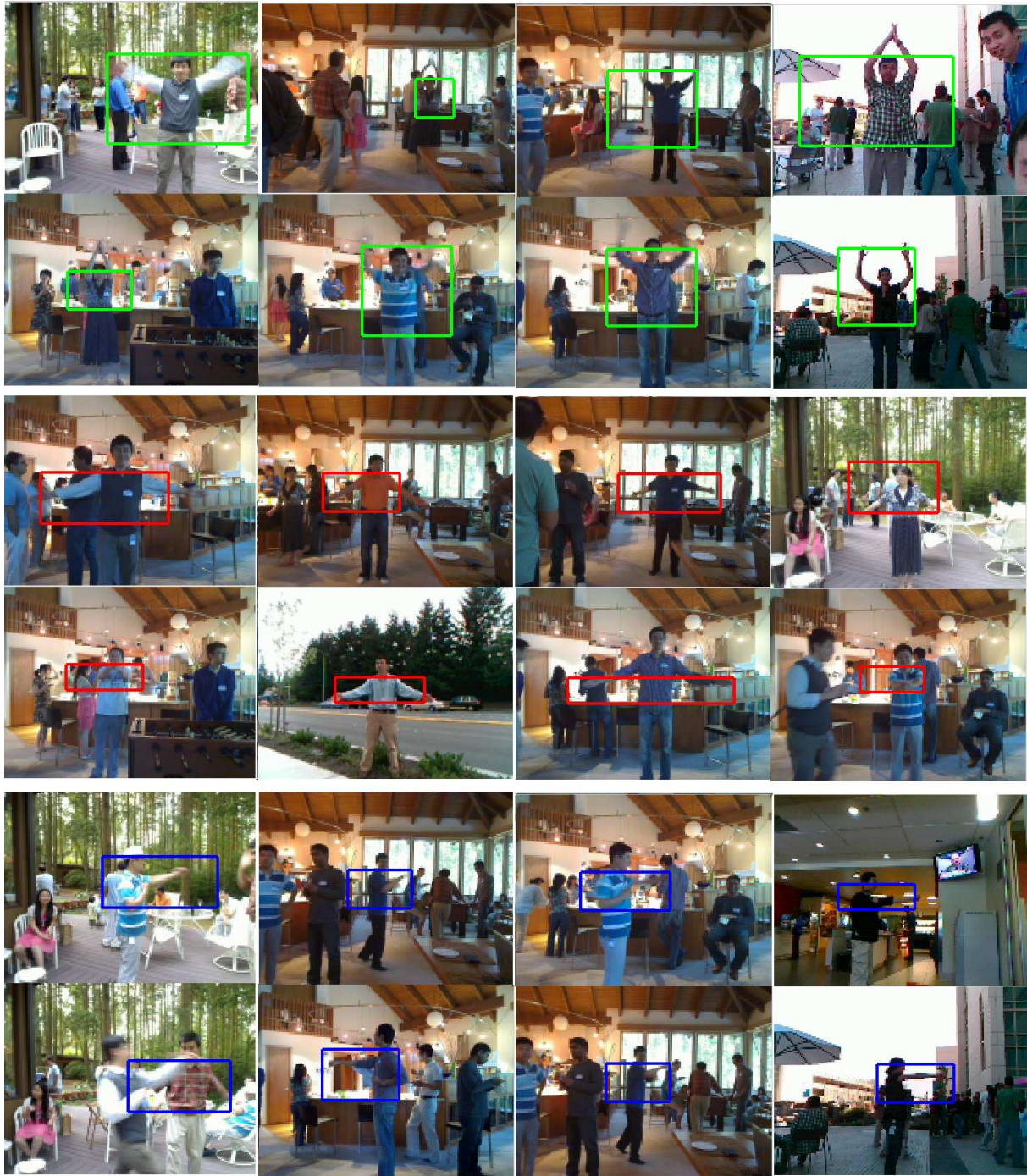
Fig. 3. Detection examples of MSR-II dataset. The bounding boxes denote the detected location using Branch-and-Bound search. The color of the bounding box denotes the action category: red for hand clapping, green for hand waving, and blue for boxing.
