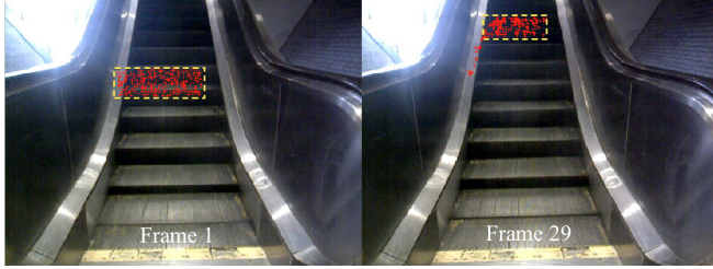
Fig. 3: Montage of Tracking Feature implemented on an upstairs escalator. The yellow box represents the region of interest selected while the red markers represent the eigenfeatures extracted from the stair.
