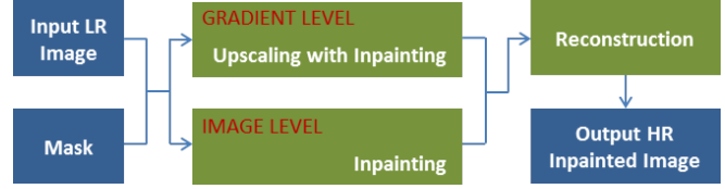
Fig. 2. Flowchart of the proposed internal exemplar-based image enhancement method. Given an input LR image with a mask indicating the missing region(s), the LR gradients are upscaled with inpainting embedded. The HR gradients, along with the inpainted LR image, are fed into an energy function to reconstruct the final HR output image.
