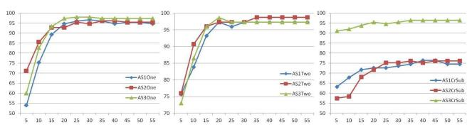
Figure 7: The recognition accuracies using different number of frames in Test One (left), Test Two (middle), and Cross Subject Test (right). 15-20 frames are sufficient to enable action recognition in most test sets.
