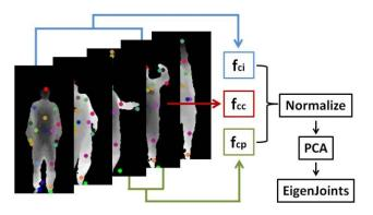
Figure 2: The framework of representing EigenJoints. In each frame, we compute three feature channels  $f_{ci}$ ,  $f_{cc}$ , and  $f_{cp}$  to capture the information of offset, posture, and motion. The normalization and PCA are then applied to obtain EigenJoints descriptor for each frame.
