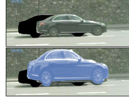
Fig. 4: Dynamic object motion disentangled image: Left is the I_{t-1}^d when depth prior is accurate. The right blue image patch shows the re-projected C_{t-1}^d with inaccurate depth prior.
