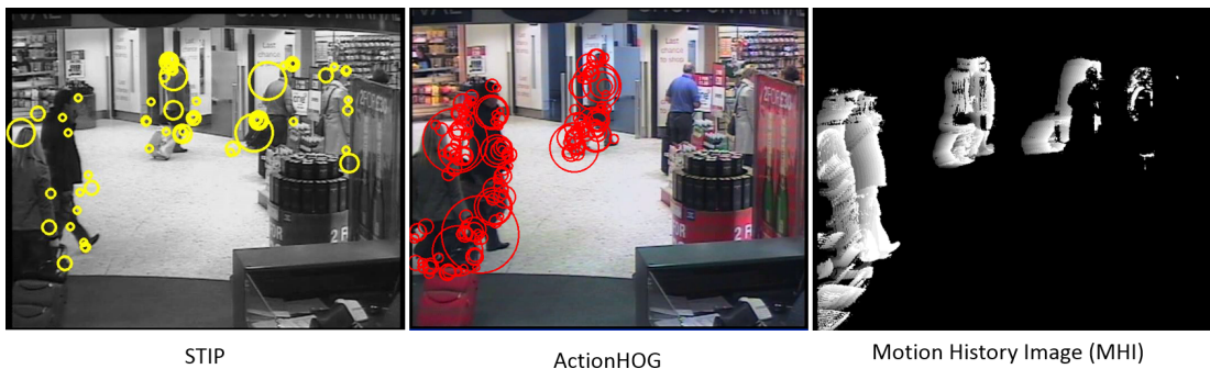
Figure 2.2: The spatio-temporal interest points detected by STIP and ActionHOG. Brighter pixels on MHI correspond to more recent motion. Gradients on MHI also provide motion direction information.
