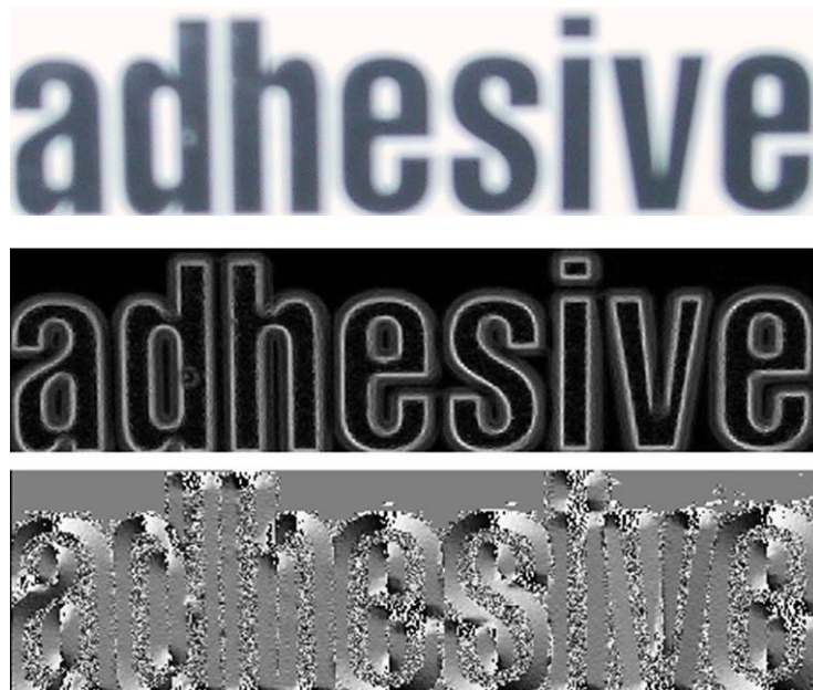
Fig. 4–4. From top to bottom, the figures represent the original text patch, the feature maps of gradient magnitude and the feature maps of gradient orientation respectively.
