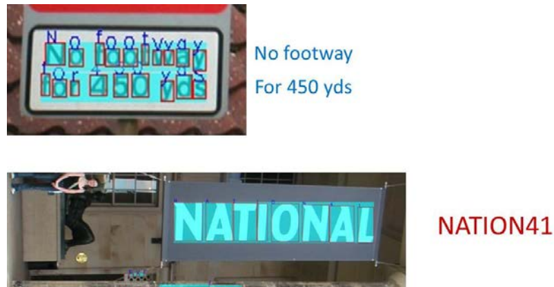
Fig. 6–1. Top row demonstrates the word recognition based on perfect STC predictions, and bottom row demonstrates the error of word recognition because of slight error of STC predictions.
