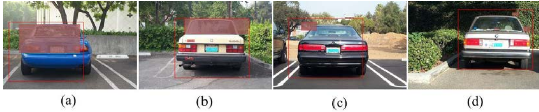
Fig. 11-3. Some post-processing examples in LP detection. Cyan regions inside red car boxes represent the true positive LP, and red regions inside red car boxes represent false positive LP detections that are filtered out by post processing.
