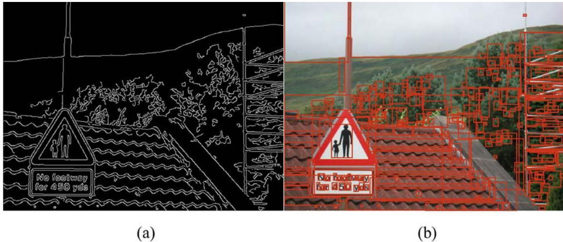
Fig. 2-5. (a) Canny edge map of a scene images. (b) Bounding boxes of all available edge boundaries in the form of connected edge pixels, obtained from edge map.
