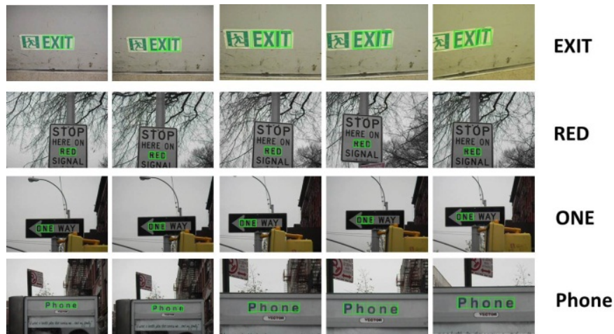
Fig. 10-2. Some example results of word recognition from multiple frames of text tracking. Right column shows recognized words.
