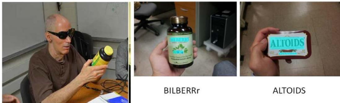
Fig. 9–4. Prototype system assists blind user read text information from hand-held objects, including the detected text regions in cyan and the recognized text codes.
