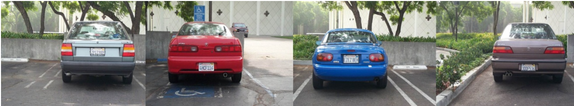
Fig. 11-1. Some examples of car-rear training samples. Each car is located at complex background. The LPs are mostly located in the central parts of car rear.
