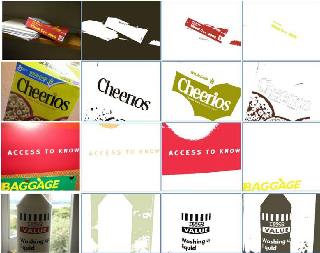
Fig. 2-2 Some examples of color-based partition, where the left column contains original images and other columns contain the corresponding dominant color layers.
