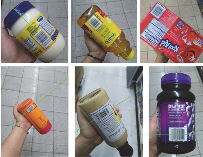
Figure 4. Successful detection results from sample images of the self-collected barcode dataset. Figure is best viewed in color.
