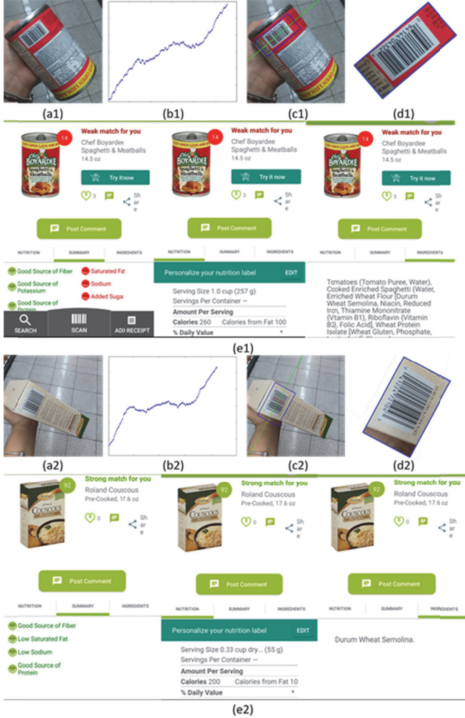
Figure 3. Illustrations of the proposed barcode detection and recognition framework on two sample images. For each instance, (a) Input image. (b) Corresponding \sigma values for the sampled pixels along the bisector line. (c) Results generated during the barcode detection step including the segment with the highest score (in red), the bisector line (in green), and the bounding box indicating the barcode region (in blue). (d) Barcode region after cropping. (e) Returned recognition results from ShopWell [14] based on the cropped barcode region. Figure is best viewed in color.
