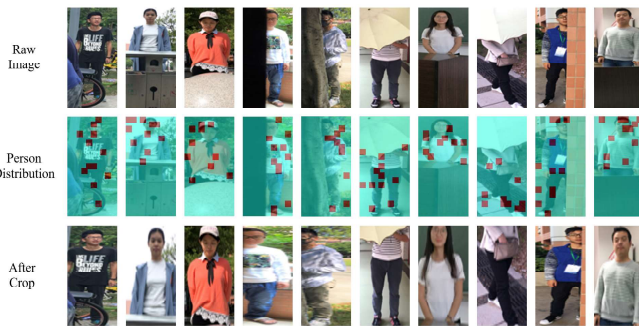
Fig. 4. The visualization of common non-occluded interest block search and MCP cropping. The top row is the raw image, the middle row is a visualization of the non-occluded region distribution of human, and the bottom row is the image after MCP cropping. The red patches in the distribution map are the human body that is highly concerned by our model. Best view in color.
