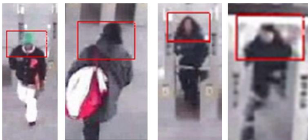
Figure 11: Sample detections in mid-field scenes, using a head and shoulders detector based on Haar features.
