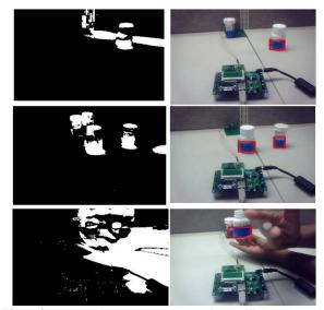
**Fig. 3:** Experiment results of medicine bottle identification by combining RFID and vision method. Left column: Foreground Images of moving objects; right column: Identifying medicine bottles by color detection. First row: Tracking of one medicine bottle. Second row: Tracking of two medicine bottles. Third row: Human action of taking out the medicine from the bottle.
