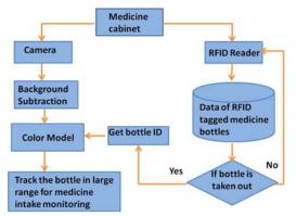
**Fig. 1:** System diagram of the proposed medicine bottle identification by combining video camera and RFID sensors.
