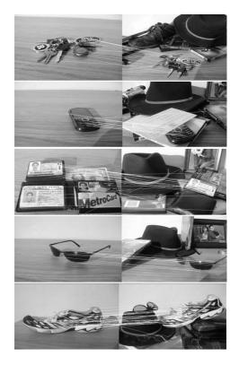
**Figure 1**: Matching between reference and test images in the presence of cluttered background under various conditions, keys (image scale), cell phone (partial occlusion), sunglasses (translation), sneaker (rotation), and wallet (change in viewpoint).
