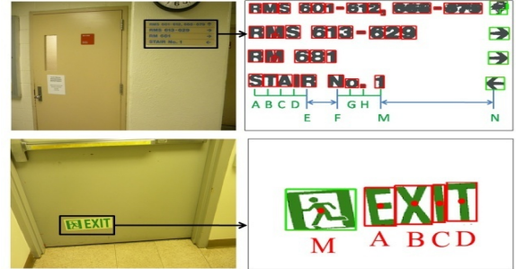
Figure 6: In the top row, the inconsistency of |EF| and |MN| leads to separation of two text strings and the arrow is filtered out; in the bottom row, area of M demonstrates inconsistency because it is much larger than its neighbors.
