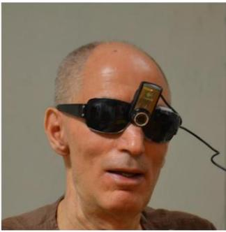
**Figure 11:** An example setup of clothing pattern recognition prototype to capture images by a web camera with auto focus on sunglasses.
