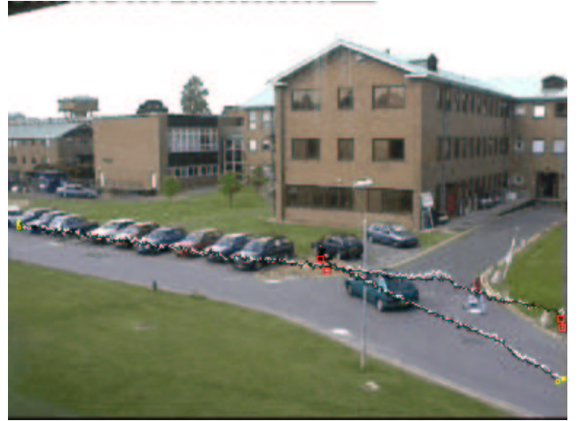
Figure 8: A comparison of estimated tracks (black) with ground truth positions (white), for two tracks superimposed on a mid-sequence frame showing the two objects.
