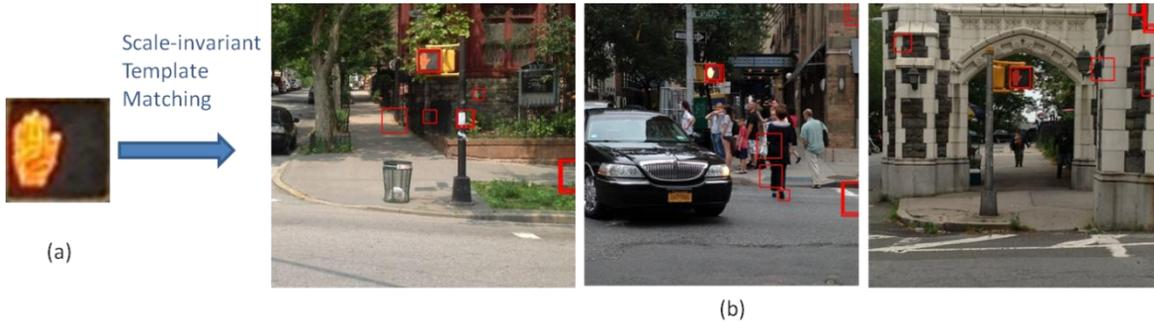
**Figure 5.** Examples of the detected candidates of crosswalk "red" traffic sign by the scale-invariant template matching. (a) Template of crosswalk "red" traffic sign; (b) detected candidates (in red boxes).
