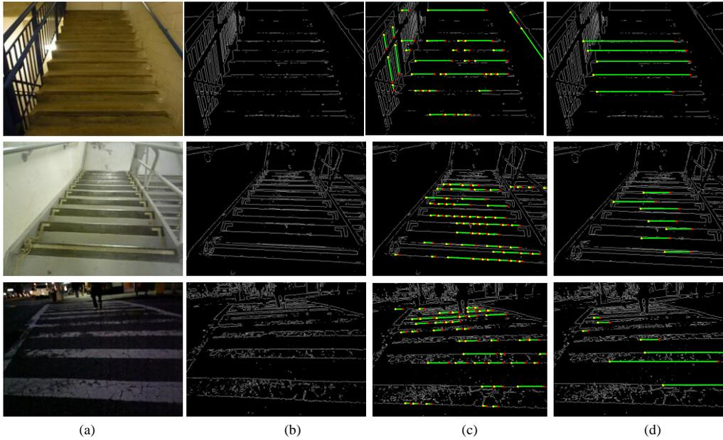
Figure 2. Example of upstairs (row 1), downstairs (row 2), and Pedestrian crosswalks (row 3). (a) Original image; (b) edge detection; (c) line detection; (d) concurrent parallel lines detection (yellow dots represent the starting points, red dots represent the ending points of the lines, and green lines represent the detected lines.)
