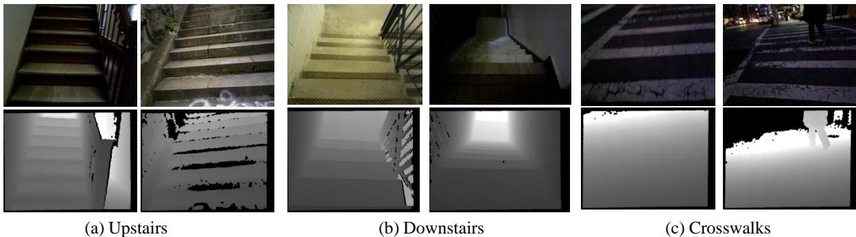
**Figure 8.** Examples of RGB (1<sup>st</sup> row) and depth images (2<sup>nd</sup> row) for (a) upstairs, (b) downstairs, and (c) pedestrian crosswalks in our database.
