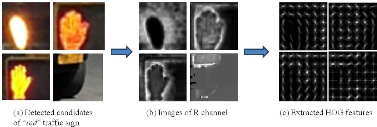
**Figure 7.** Extracting HOG features for the detected candidate regions of crosswalk "red" traffic sign from the Red channel.
