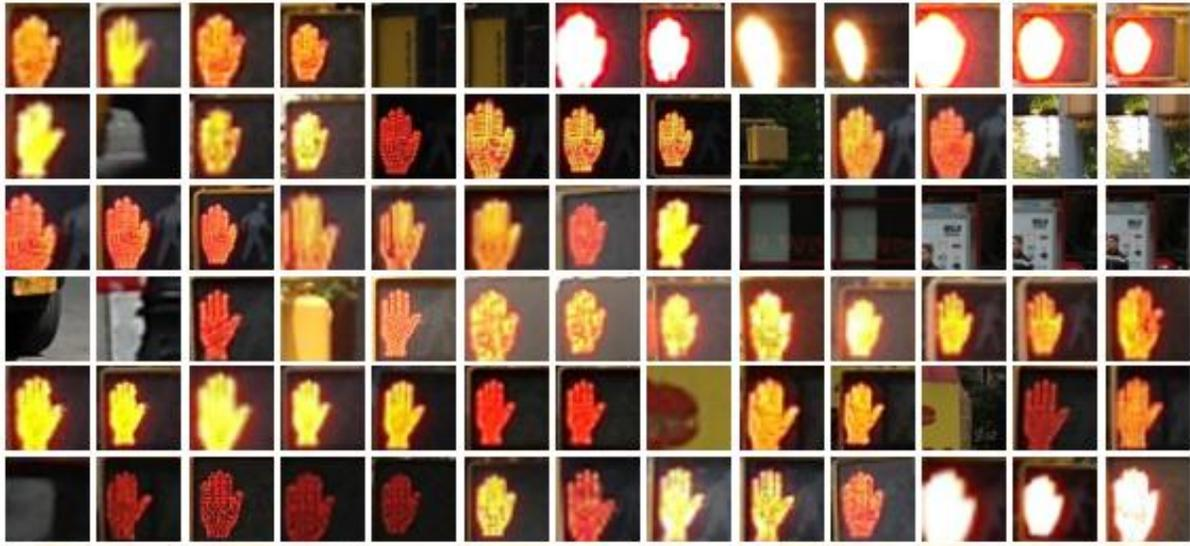
**Figure 6.** Examples of the detected candidates of crosswalk "red" traffic sign by the scale-invariant template matching and color segmentation.
