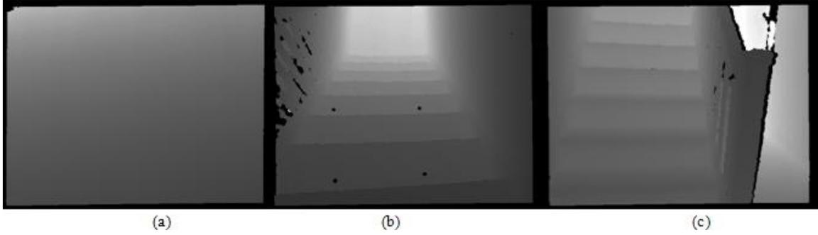
**Figure 3.** Depth images of (a) pedestrian crosswalks, (b) downstairs, and (c) upstairs.
