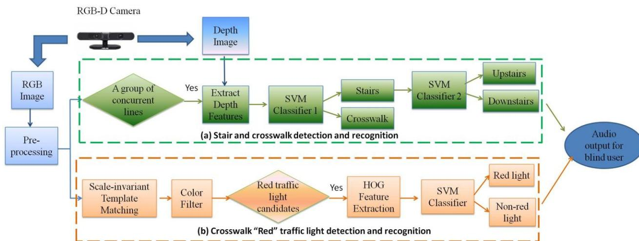
**Figure 1.** Flowchart of the proposed algorithm for stair, pedestrian crosswalk, and crosswalk "Red" traffic sign detection and recognition.
