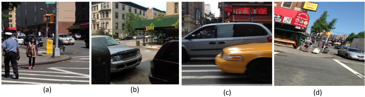
**Figure 13.** Examples of our proposed method of "red" crosswalk traffic sign recognition fails. (a) Image with low contrast between the changes of "red" and "walking" signs; (b) image with large camera view angle change; (c) image with occluded crosswalk traffic sign by passing vehicles or pedestrians; (d) image with large camera rotation.
