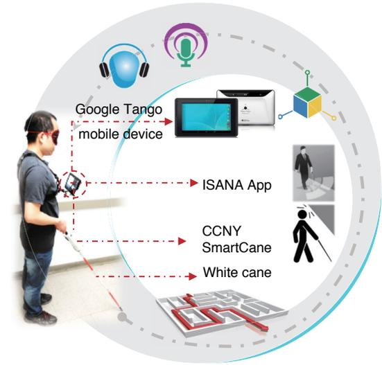
Fig. 2. ISANA and SmartCane system configuration on a blindfolded sighted subject
