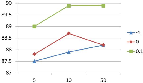
Figure 6. Performance evaluation of E<sup>2</sup>DMM on dynamic hand gesture dataset [9] of different parameter settings. X axis: penetration threshold  $\epsilon$ ; Y axis: performance in term of classification accuracy. Blue, red and green colored curves indicate degree of enhancement -1, 0, and 0.1 respectively. Notice that when degree of enhancement is -1, it actually represents traditional DMM [16].
