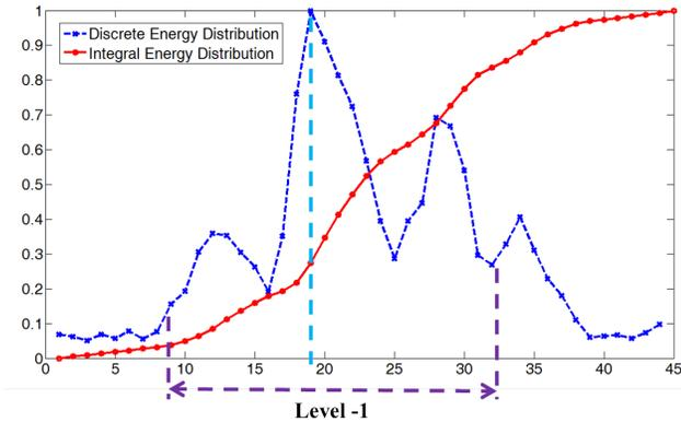
Figure 5. Illustration of how to dynamically select “level -1” based on the energy distribution over time. Blue curve shows the energy of each frame. Red energy shows the integral energy over time. Cyan dashed line shows the frame with highest energy and purple dashed line shows the chosen window for “level -1”. X-axis is frame index and Y-axis is the relative magnitude of each curve.
