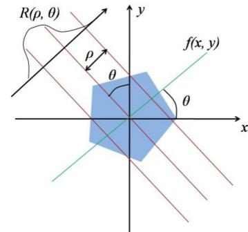
Figure 2. Radon transform of an image  $f(x, y)$ .
