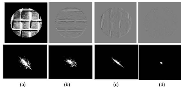
Figure 7. Co-occurrence matrices: (a) Input image & co-occurrence matrix; (b) Horizontal Wavelet & co-occurrence matrix; (c) Vertical Wavelet & co-occurrence matrix; (d) Diagonal Wavelet & co-occurrence matrix.
