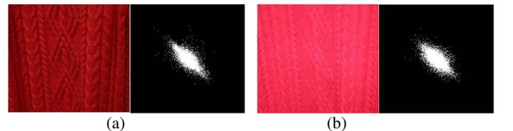
Figure 10. Our method handles illuminations changes. (a) Image 1 of a sweater and the corresponding co-occurrence matrix; (b) image 2 of the same sweater with large lighting change and the corresponding co-occurrence matrix. The distance between the image pair is very small and the image pair is detected as "match".
