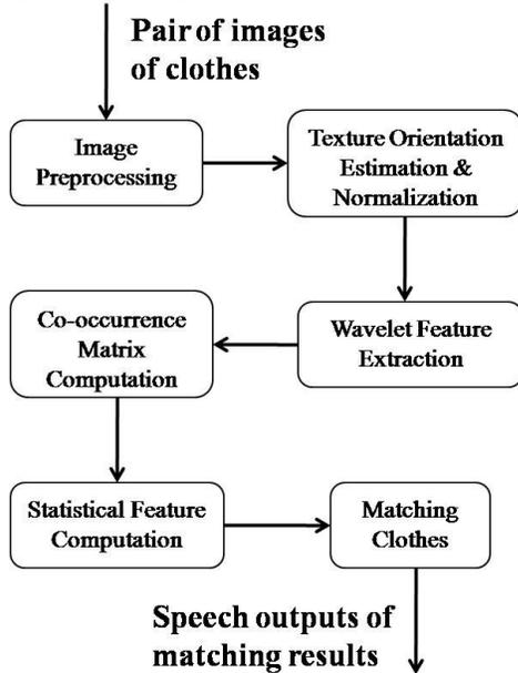
Figure 1. System diagram of matching clothes with complex patterns for blind people
