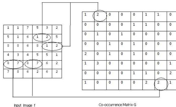
Figure 6. An example of a size 8\*8 co-occurrence matrix by considering a pixel and its right neighbor. Element  $G(1, 2)$  is 2 because there are two occurrence in image  $f$  of a pixel valued 1 having a pixel valued 2 immediately to its right. Element  $G(8, 7)$  is 2 because there are 2 occurrences in  $f$  of a pixel with value of 8 having a pixel valued 7 immediately to its right.
