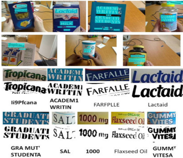
Figure 10. The top two rows present some results of text localization on the blind-captured dataset, where localized text regions are marked in cyan. The bottom rows show two groups of enlarged text regions, binarized text regions and word recognition results from top to down.
