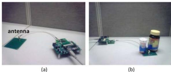
**Fig. 2:** SkyTek M2 RFID system [3] includes USB connection, antenna, reader and a host interface board for identifying medicine bottles.
