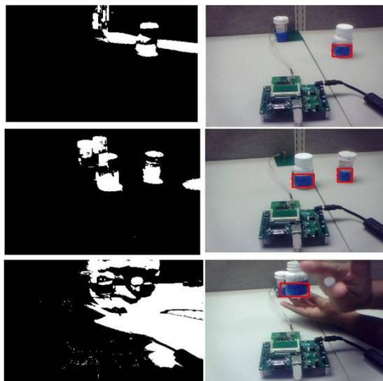
**Fig. 3:** Experiment results of medicine bottle identification by combining RFID and vision method. Left column: Foreground Images of moving objects; right column: Identifying medicine bottles by color detection. First row: Tracking of one medicine bottle. Second row: Tracking of two medicine bottles. Third row: Human action of taking out the medicine from the bottle.
