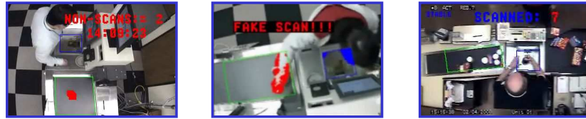
Fig. 7. Fake-scan action detection results with different check-out lanes and different camera settings. First keyframe captures the number of fake-scans. Middle keyframe captures a particular fake-scan action. Last keyframe shows the total number of scan actions captured.
