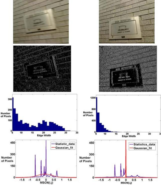
Figure 5. The edge width and MSCN distribution for the blurred (left column) and unblurred (right column) frames. In the two examples, from top to bottom, there are original images; edge width distributions, edge images, and MSCN distributions.
