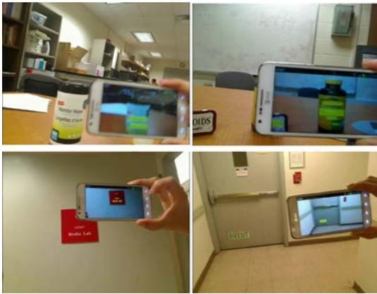
Figure 7. The demo system of text extraction runs on a smart phone with Android platform.
