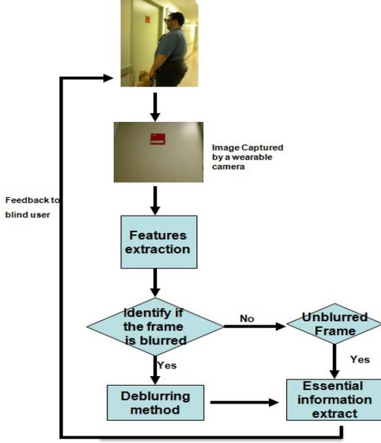
Figure 3. The flowchart of the proposed method for detecting good quality frames from blurred frames from videos captured by a wearable camera.
