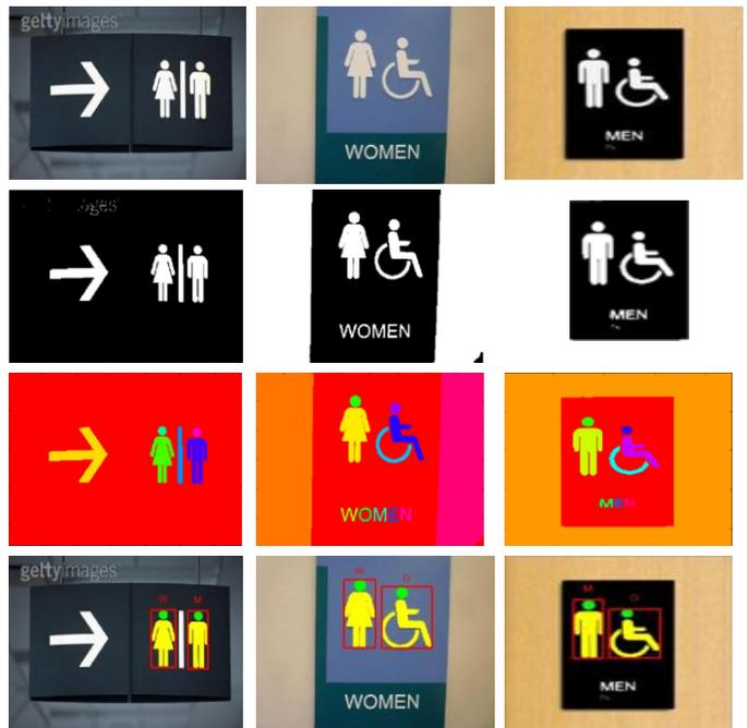
Figure 9. Sample restroom signage images of each step of the proposed method. Rows from top to bottom: original images, binarized images, images with connected components, and detected and recognized signage.
