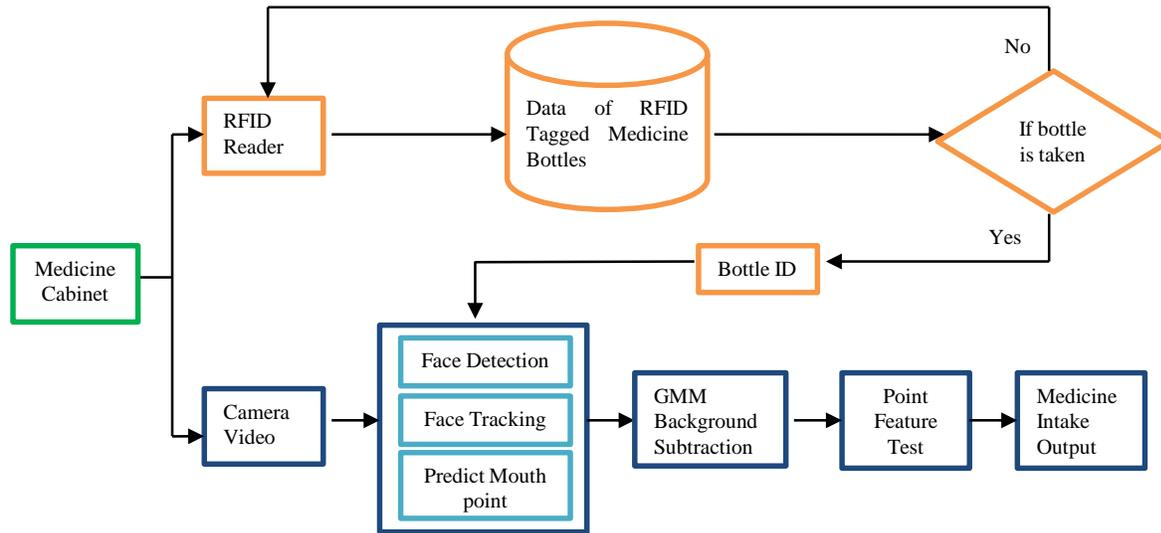
Figure 1. System diagram of the proposed medicine bottle identification by combining video camera and RFID sensors.
